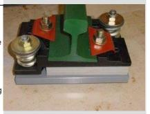
The resilient pad consists of an elastomer that has a low dynamic to static spring rate and excellent electrical resistance and thermal stability. The dynamic stiffness of the system can be as low as 5 kN/mm (at 20 Hz), ensuring a first wheel-rail vertical resonance below 20 Hz and hence excellent vibration isolation characteristics, comparable to those of the floating slab.
